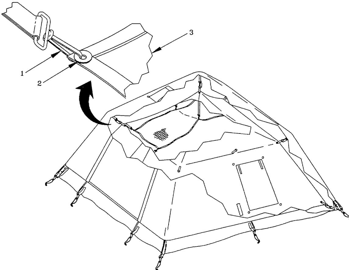
From inside the tent body or liner (if used) on the side opposite the stovepipe shield, attach snap hooks (1) on side, front and back corners, and center of tent to grommets (2) on edges of gear loft (3).
