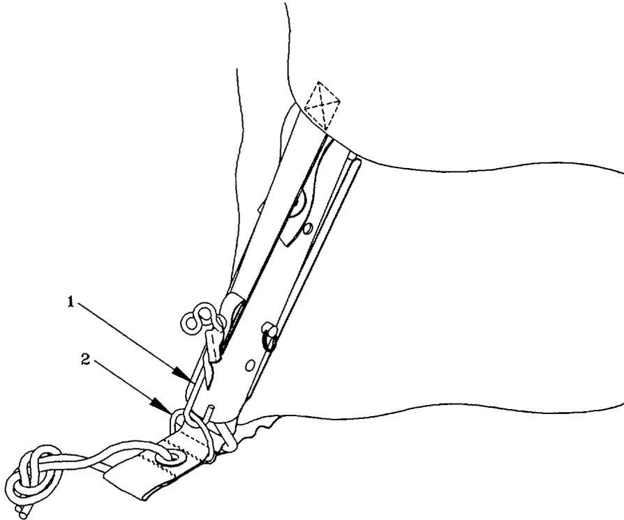
Stake corners of tent through rope buckets (1), using tent pins (2). Square and tension floor before driving tent pins at a 15 degree angle towards the tent. Repeat staking at center of tent sides. Adjust tension of fly by loosening or tightening webbing through adjustable hooks.
