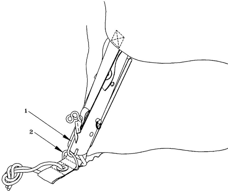
(4) Secure adjustable hooks (1) on fly assembly to dee (D) rings (2) at corners of tent.
