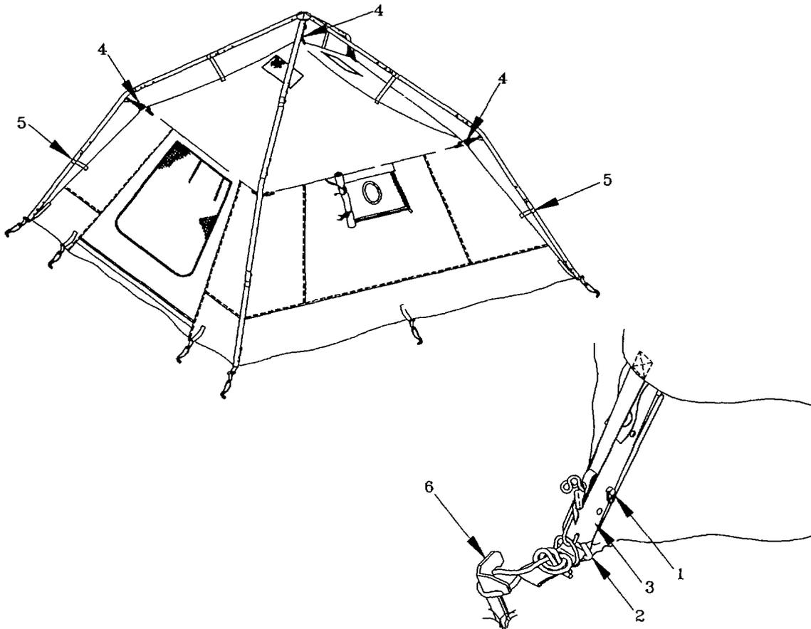
Step 1. Check frame assembly for proper setup, loose or missing hardware (1). Check that floor to frame connectors (2) are installed in bottom of frame poles (3).
