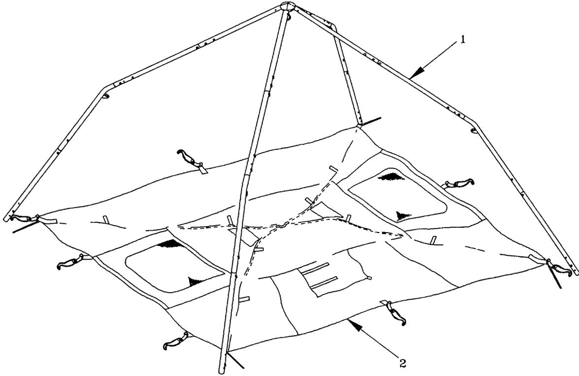
(6) Position assembled frame (1) over tent body assembly (2), with end sections of legs at tent corners.
