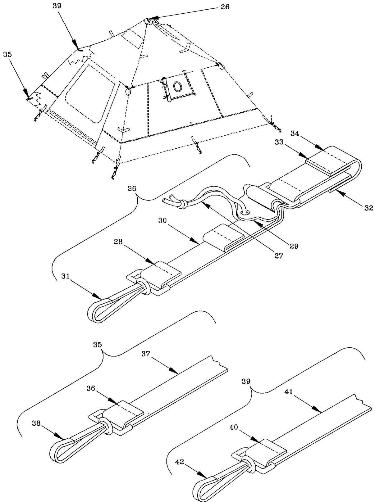
Figure 2. Tent Body Assembly (Sheet 2 of 7)
