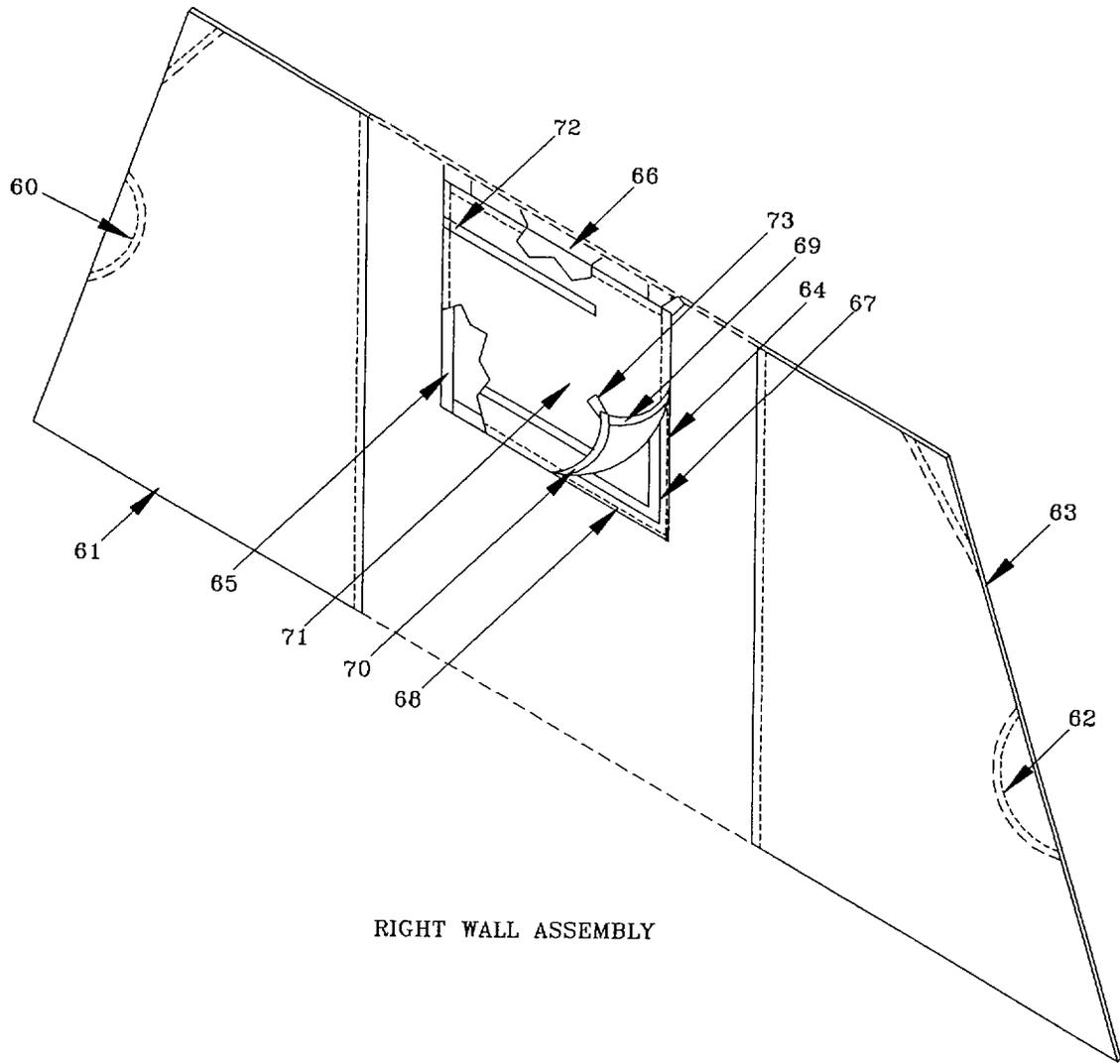
Figure 2. Tent Body Assembly (Sheet 5 of 7)
