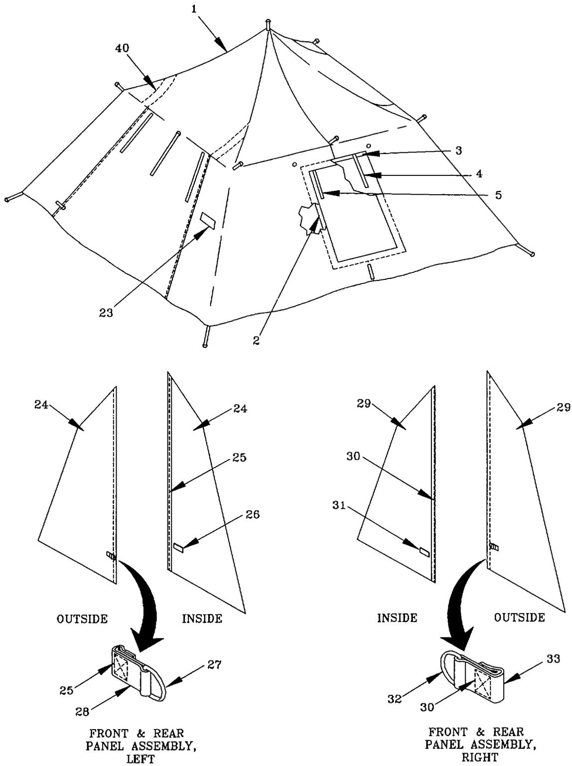
Figure 4. Liner Assembly (Sheet 1 of 2)
